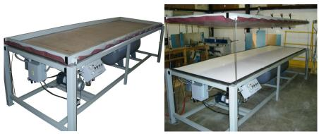
posal and there is a vacuum control switch so the pump only runs when it is need. There is a release button to clear the vacuum in the forming area quickly. It's very easy to use.
